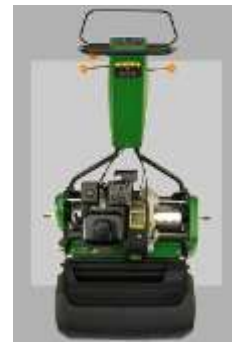
Figure 2 A 22" John Deere hybrid greens mower with electric reel drive.
